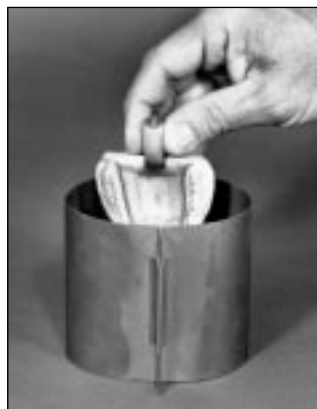
Figure 29: WAX PATTERN facing toward seam of flask former
