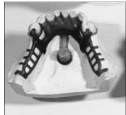
Figure 20: TYPICAL SINGLE SPRUING from bulky to smaller volume areas
