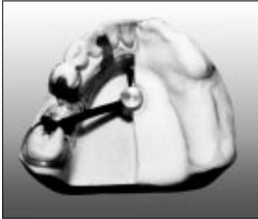
Figure 32: PAINT-ON INVESTMENT with an "even layer" of approx. 1/8"
