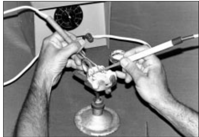
Figure 49: CARBON GROUND AND SOLDER IN POSITION
