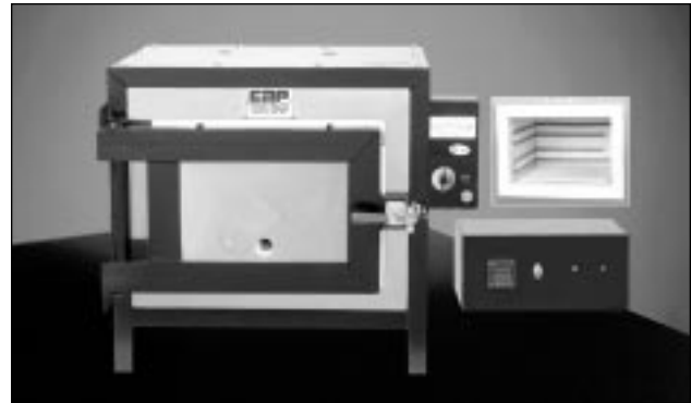
Figure 41: 18 CASE ELECTRIC BURNOUT FURNACE
