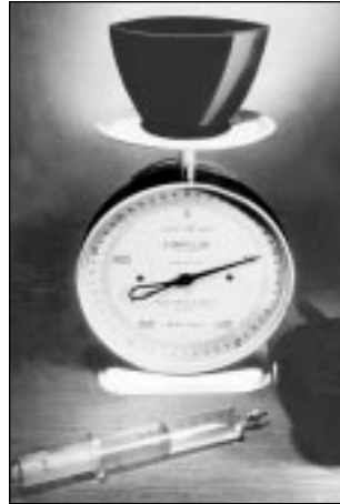
Figure 12: CAREFULLY WEIGH investment and measure water for accuracy
