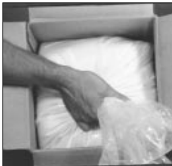
Figure 14: SQUEEZE AIR out of investment bag to prevent contamination
