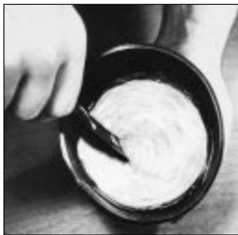
Figure 36: HAND SPATULATE for 60 seconds
