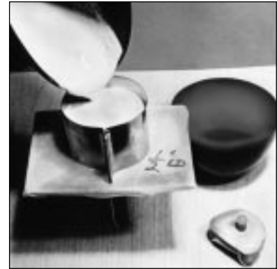
Figure 37: FILL FLASK 3/4 FULL with investment
