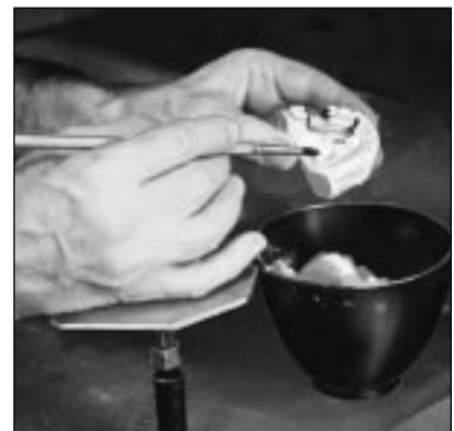
Figure 31: VIBRATING PAINT-ON INVESTMENT "ahead of the brush" with a thin, uniform thickness
